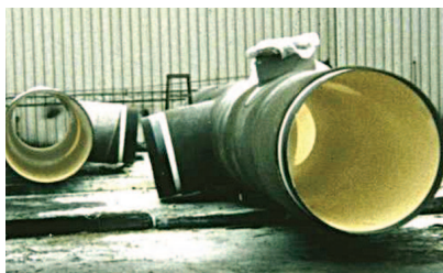
Figure 8: The application of a highly abrasion resistant 100% solids rigid polyurethane lining on a 36" steel pipe for extremely high water flow rate.
